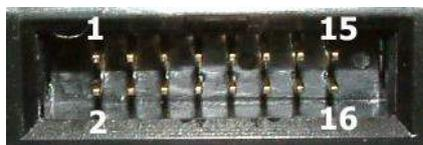
When a Payout, Ticket Module or Docking Plate is connected a 16-pin Molex 0039012165 connector will replace the 16-pin Molex 9733272, the Pinout is below:
