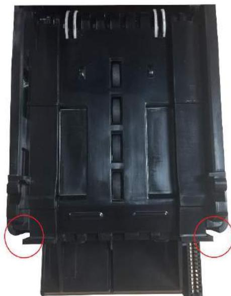
3. **Carefully but firmly push the BNF down onto the UAP so that the connectors dock together.**
