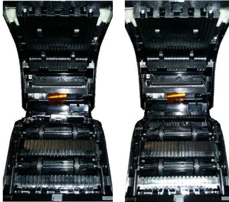
Part of the SMART Ticket needs to be removed so the whole path can be cleaned. The PM01018 is used to guide the paper, the part is shown in situ below.
