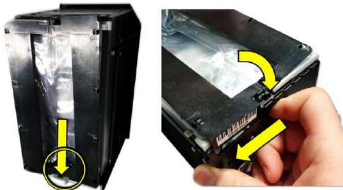
Slide the cash bag back into the TEBS and turn the lock – the lock will go red. The stacker will audibly cycle and the bezel flash code will disable showing the barcode has been read.
