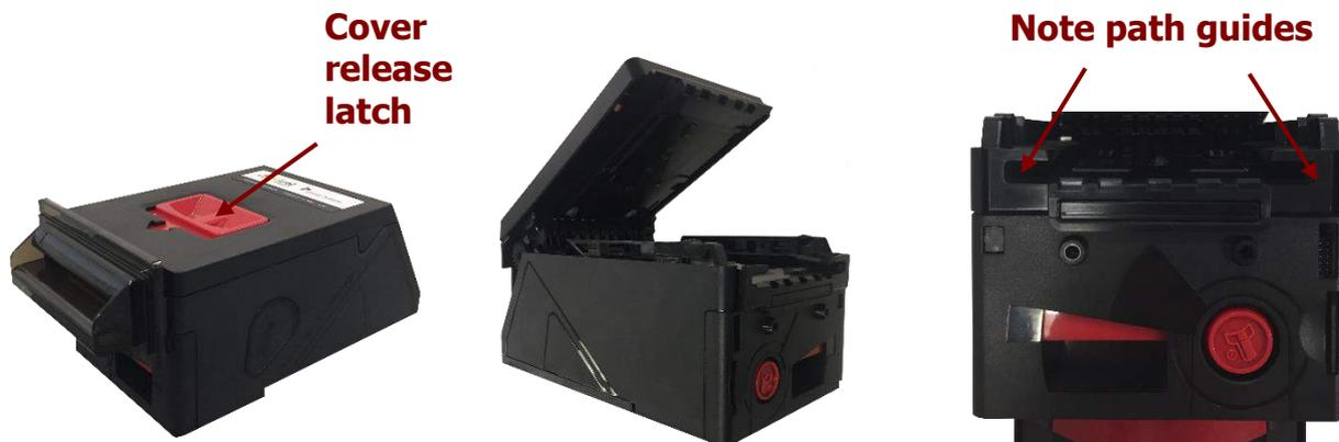
The note path is visible and can be cleaned. Carefully wipe the surfaces with a soft lint free cloth that has been dampened (NOT wet) with a water and mild detergent solution (e.g. household washing up liquid) - be very careful when cleaning around the sensor lenses and make sure they are clean and dry before closing the cover and powering the unit.
