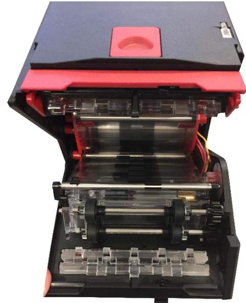
Notes can now be removed from both areas where visible. Once the notes are removed follow the next step to ensure that tapes are properly tensioned.
