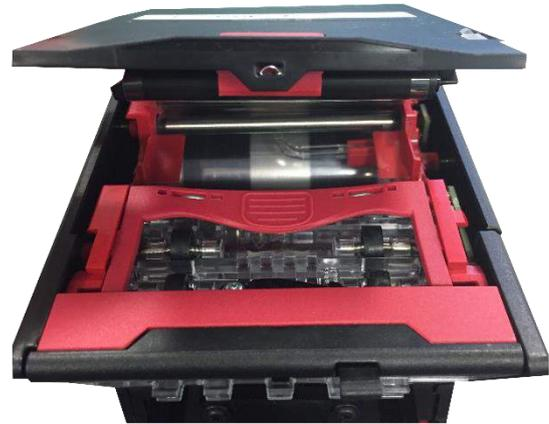
To open the second door, press the red latch inside the first door as per the picture below. The second door will spring open:
