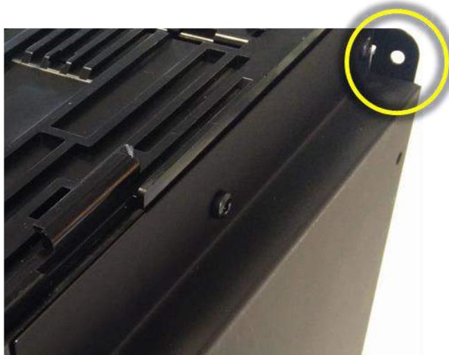
Lack of proper bonding can cause communication issues and other failures. The resistance between the chassis and Earth should be less than 0.7Ω.
