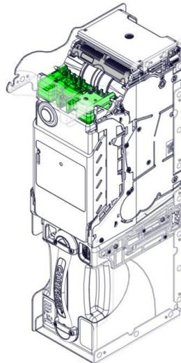
**Chassis** - metal frame containing all the other modules. The Recycler Module is permanently fixed to the chassis.
